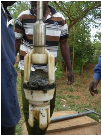
Clayey material on the handpump plunger caused by siltation
